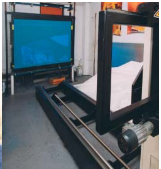
Miniature film is projected on to a photo-sensitive screen
